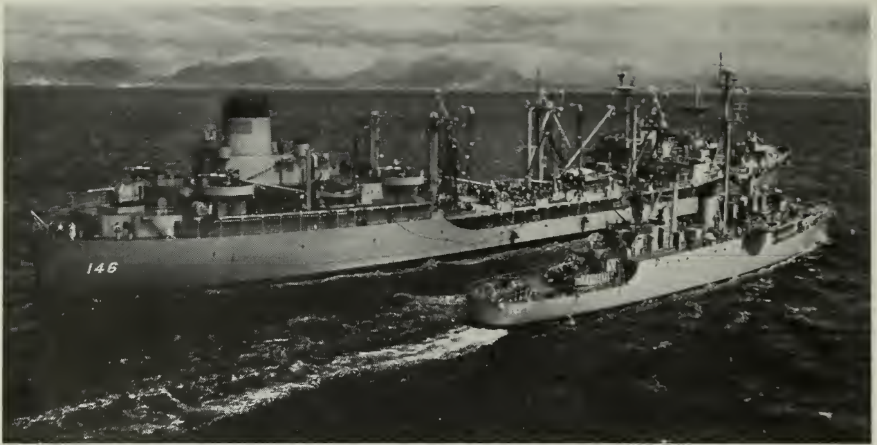
SIDE BY SIDE—USS Kawishiwi (AO 146) pipes load of NSFO to USS Fessenden (DER 142) while in Hawaiian waters.
